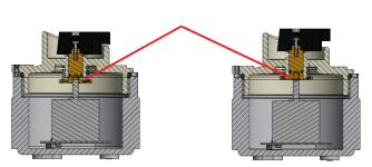
c. Turning CCW door while holding out rotary handle
