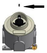
b. Pull out rotary handle 4mm (it stops after this course mechanically) and hold it
